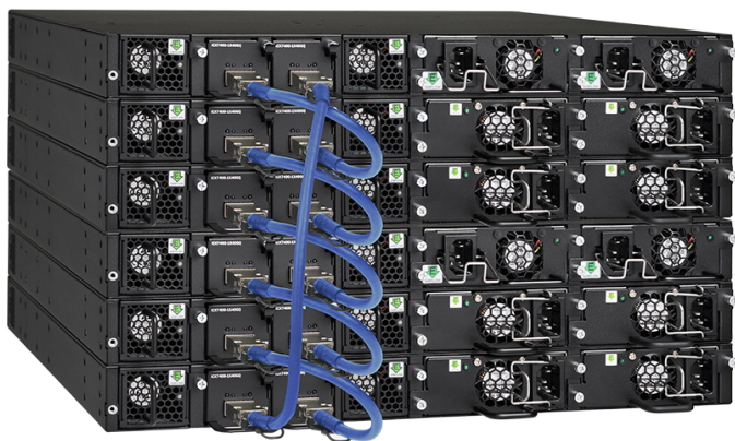
Figure 1: Ruckus ICX switches can be stacked together using standard SFP+ or QSFP+ ports and optics to create a single logical device over distances up to 10 km.
